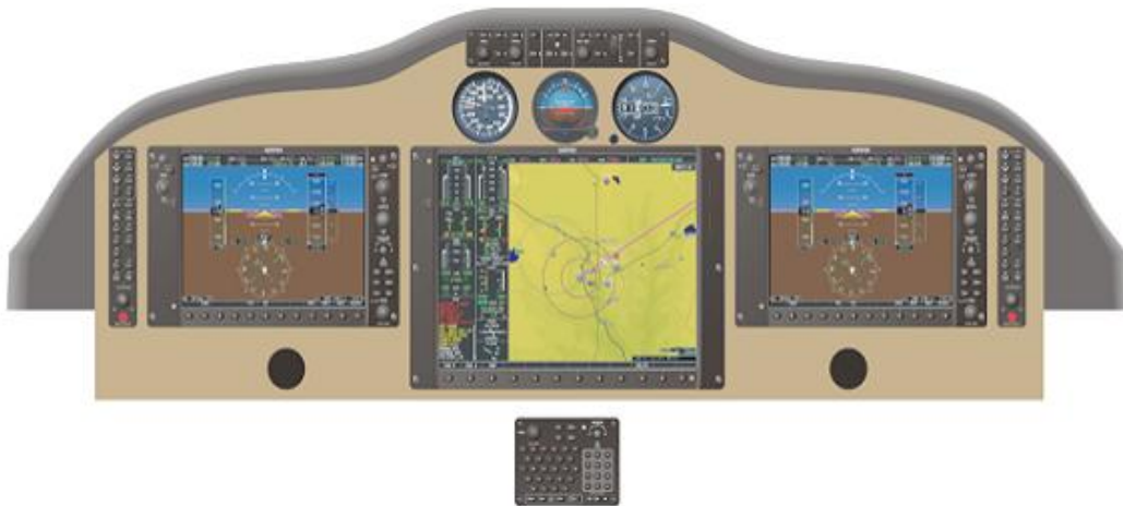
Figure 2-6 Three Display Installation (Example)
