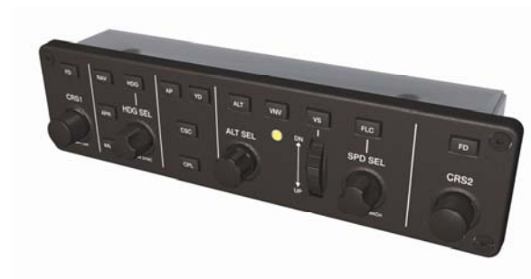
Figure 3-17. GMC 715 AFCS Control Unit
