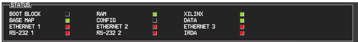
Figure 4-8. Data Transmission Indicators
