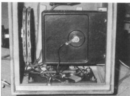
Figure 5. Another underside view with the tuning capacitor in place.
