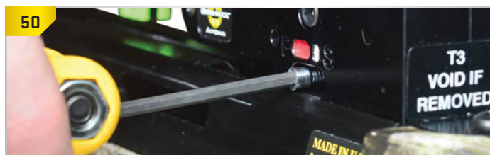
Remove the hex-head cap screw.
