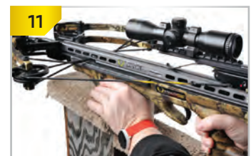
11 Keep your thumb and fingers below the flight deck and away from the cables to avoid injury.
