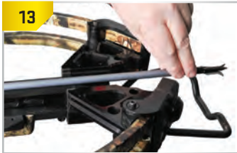
13 PROPER HAND POSITION. Hold the arrow with your index and middle finger and your thumb just behind the broadhead.
