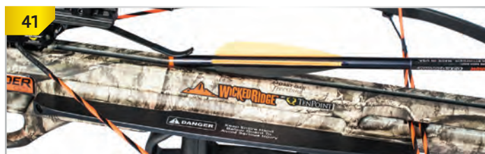
41 Insert one of the vanes into the barrel's flight groove.
