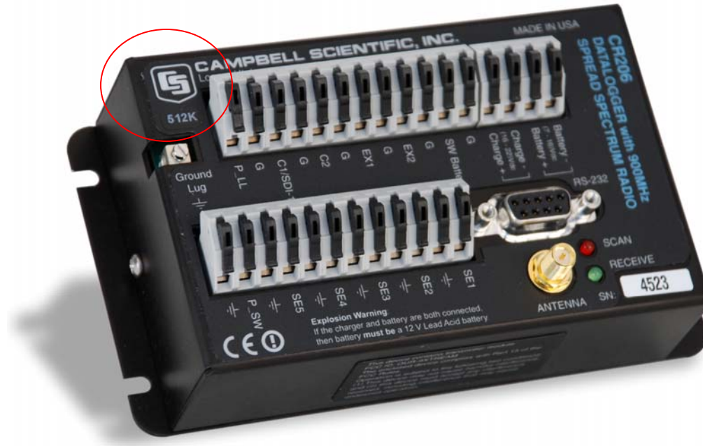
FIGURE OV2-1. 512K on the datalogger label indicates the larger memory.
