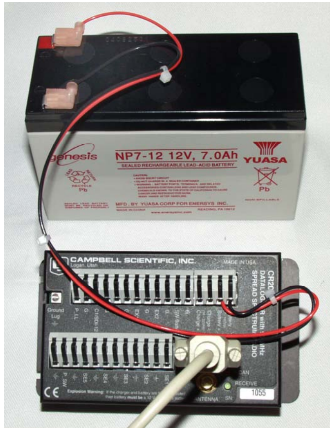
FIGURE OV3-1. Power and Communication Connections to the CR200
