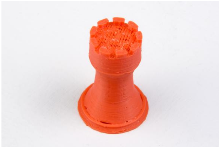
Figure 2.15: An example of insufficient top layers.
