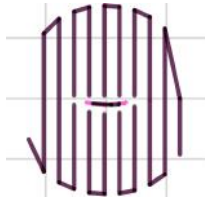
Figure 2.39: Support infill pattern: Rectilinear
