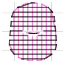
Figure 2.40: Support infill pattern: Rectilinear Grid
