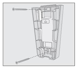
■ Attach the mounting plate to the wall.
