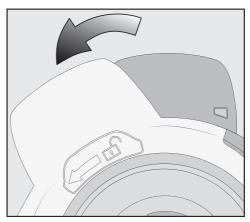
■ Turn the lid of the dust container in the direction of the arrow as far as the first stop.
