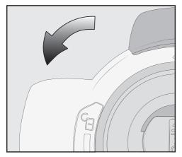
■ Turn the lid of the dust container in the direction of the arrow as far as the next stop.
