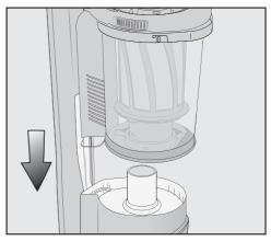
■ Slide the dust container handle along the guide line and down on to the PowerUnit connector from above until it audibly clicks into place.
