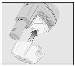
Push the battery along the guide lines until it audibly clicks into place in the PowerUnit.
