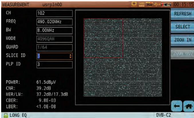
Figure 7: DVB-C2 4096QAM Constellation
