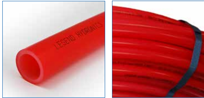
The externally-extruded EVOH oxygen barrier reduces oxygen molecule permeation into the water. Compliant with standard DIN4726(<0.1 grams/m 3 /day)
