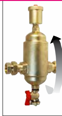
To maximize air removal, the larger half of the bowl should be on top.
