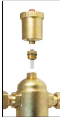
The automatic High Capacity Air Vent attaches to the T-88 through a check valve to allow removal without system pressure loss.
