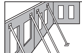
TILT-UP WALL PANELS
