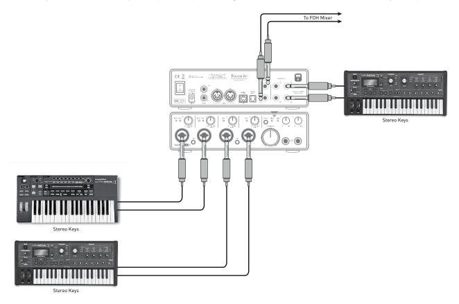
In the example illustrated, three stereo keyboards are connected to the inputs of the Scarlett 18i8; the Monitor Outputs go to the main PA system. The performer can adjust the volume of two of the keyboards against the third from the front panel; he/she can also adjust the overall level of the keyboard mix.
