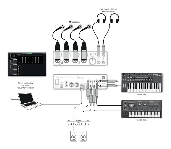
When using Direct Monitoring, ensure that your DAW software is not set to route any inputs (what you are currently recording) to any outputs. If it is, the musicians will hear themselves "twice", with one signal audibly delayed as an echo.
