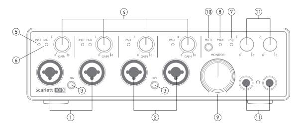
The Front Panel includes input connectors for Mic, Line and Instrument signals, the input gain and monitoring controls, and sockets for headphones.
