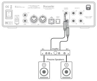
All the line output connectors are 3-pole (TRS) ¼" (6.35 mm) jack sockets, and are electronically balanced. Typical consumer (hi-fi) amplifiers and small powered monitors will probably have unbalanced inputs, either on phono (RCA) sockets, or via a 3.5 mm 3-pole jack plug intended for direct connection to a computer. In either case, use a suitable connecting cable with jack plugs at one end.
