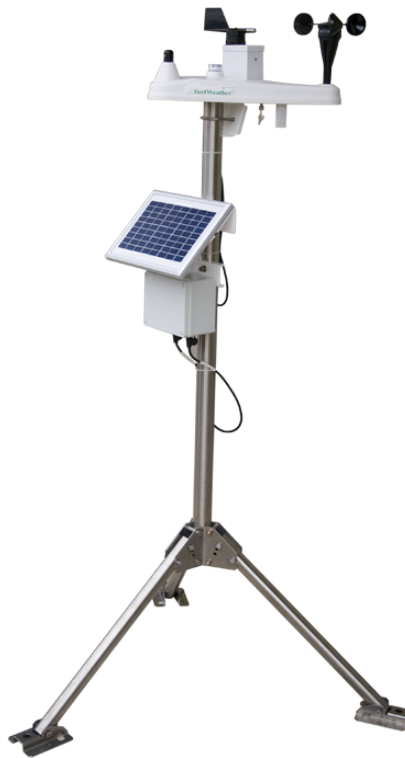
FIGURE 5-16. Short haul enclosure mounted to the 16776 tripod
