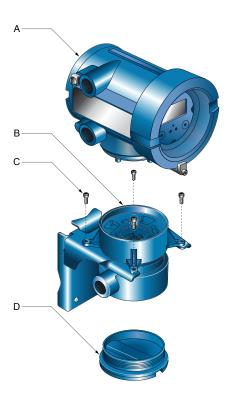
Figure 10-2: 9-wire remote installation components
