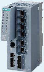
Industry uses the Power over Ethernet (PoE) technology known from office and home applications and adds the Scalance XC-200PoE, XR-100PoE WG, and XR-300PoE WG Industrial Ethernet switches to the Scalance X family portfolio. PoE switches that are suitable for powering surveillance cameras, Scalance W IWLAN Access Points, Simatic RTLS Gateways, and Simatic MV500 optical identification systems are now available for the entire industrial network.
