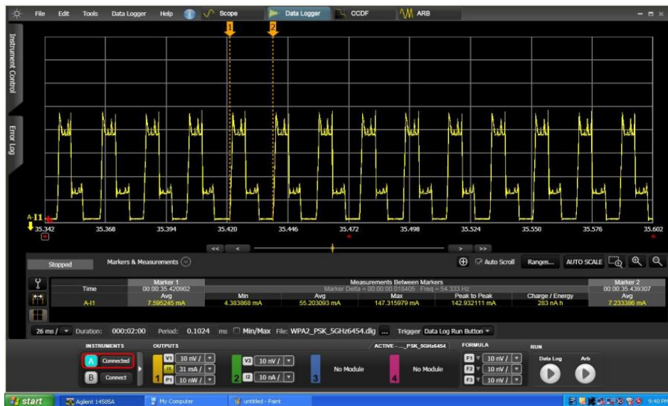
Figure 17: Power Profile in the Connected State
