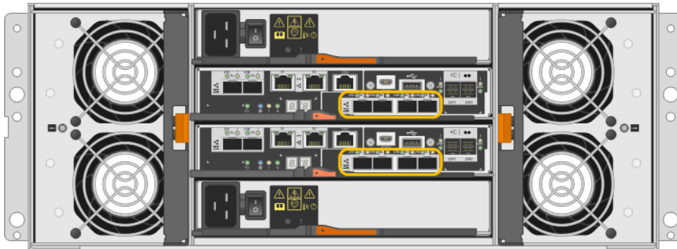
Figure 29. With two 4-port SFP+ (optical) HICs (4U)
