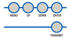
**MENU:** Used to enter menu mode and to navigate back within the menu structure.
