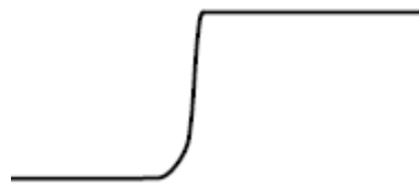
Signal with a short ground lead
