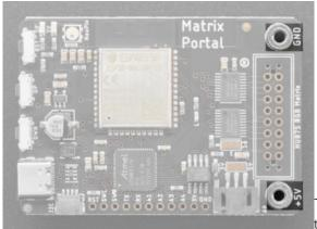
There are **+5V** and **Ground** screw terminals on either side of the HUB75 connector. These provide power to the RGB Matrix.
