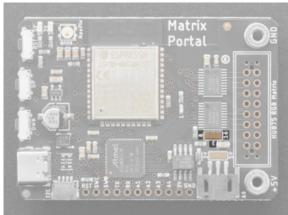
This jumper is used for use with **64x64 matrices** and is either connected to pin 8 or pin 16 of the HUB75 connector. Check your matrix to see which pin is used for address E.
