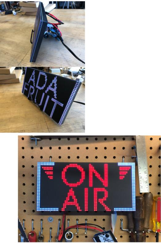
Alternately, you can use a frame, 3D printed brackets (https://adafru.it/MZf), tape, glue, or even large binder clips to secure the acrylic to the sign and then mount it on on a wall, shelf, or display cabinet.
