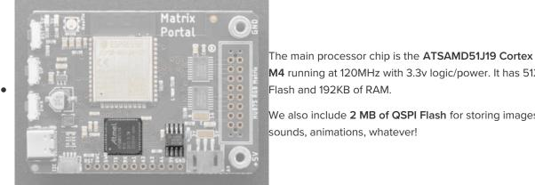
M4 running at 120MHz with 3.3v logic/power. It has 512KB of Flash and 192KB of RAM.
