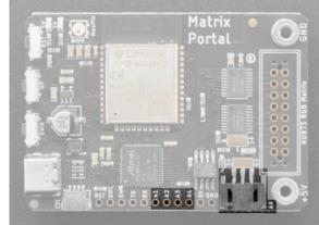
On the bottom side towards the right, there is a connector labeled **A0**. This is a **3-pin JST analog connector** for sensors or NeoPixels, analog output or input
