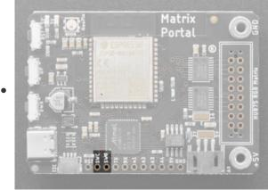
If you'd like to do more advanced development, tracedebugging, or not use the bootloader, we have the SWD interface exposed.
