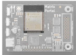
The WiFi capability uses an **Espressif ESP32 Wi-Fi** coprocessor with TLS/SSL support built-in.
