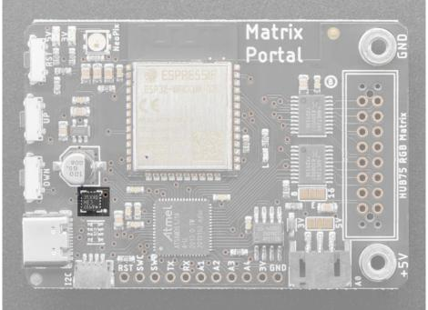
On the back of the MatrixPortal is a triple-axis accelerometer that you can use to detect motion. (That's how our cool digital sand demo works!)
