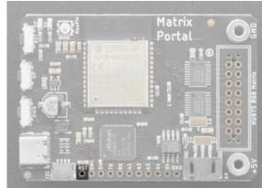
**RST** is the Reset pin. Tie to ground to manually reset the ATSAMD51, as well as launch the bootloader manually.
