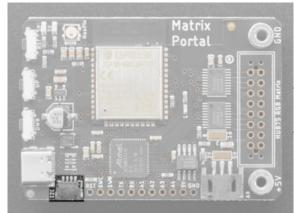
There is a 4-pin **Stemma QT connector** on the left. The I2C has pullups to 3.3V power and is connected to the LIS3DH already.
