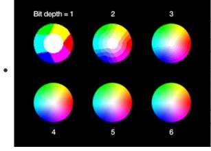
The effect of bit depth on image quality. Color values are always specified as full 16-bit "565" values, but will quantize to coarser representations at lower bit depths.
