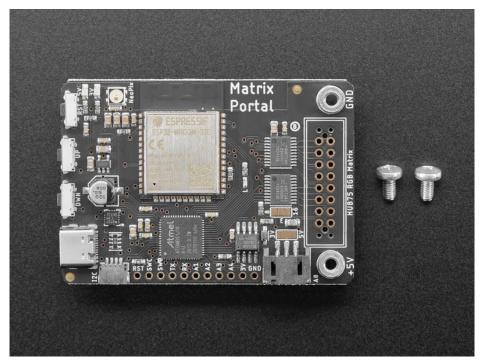
The Matrix Portal uses an ATMEL (Microchip) ATSAMD51J19, and an Espressif ESP32 Wi-Fi coprocessor with TLS/SSL support built-in. The M4 and ESP32 are a great couple - and each bring their own strengths to this board. The SAMD51 M4 has native USB, so it can show up like a disk drive, act as a MIDI or HID keyboard/mouse, and of course bootload and debug over a serial port. It also has DACs, ADC, PWM, and tons of GPIO, so it can handle the high speed updating of the RGB matrix.
