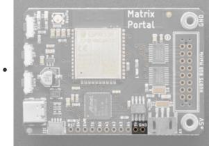
**3V** is the output from the 3.3V regulator, it can supply 500mA peak.
