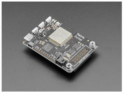
Plug The Matrix Portal directly into the back of any HUB-75 compatible display (all the ones we stock will work) from 16x32 up to 64x64 (https://adafru.it/NAX)! Use the included screws to attach the power cable to the power plugs with a common screwdriver, then power it with any USB C power supply. (For larger projects, power the matrices with a separate 5V power adapter)
