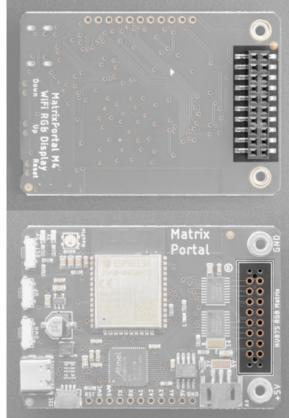
There is a **2x8 pin HUB75** connector on the reverse side that plugs directly into the HUB75 port on your RGB Matrix.
