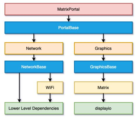
There are two main branches of dependencies related to Network Functionality and Graphics functionality. The **MatrixPortal** library ties them both together and allows easier coding, but at the cost of more memory usage and less control. We'll go through each of the classes starting from the bottom and working our way up the diagram starting with the Network branch.
