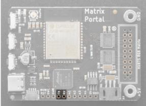
The **TX pin** and **RX pin** are for serial communication with the SAMD51 microcontroller and can be used to connect various peripherals such as a GPS.
