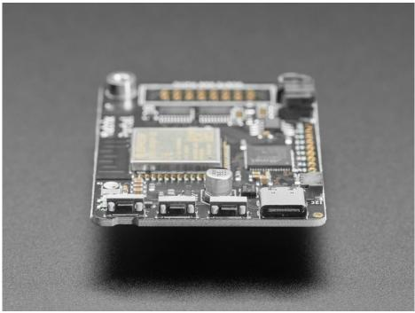
Meanwhile, the ESP32 has secure WiFi capabilities, and plenty of Flash and RAM to buffer sockets. By letting the ESP32 focus on the complex TLS/SSL computation and socket buffering, it frees up the SAMD51 to act as the user interface. You get a great programming experience thanks to the native USB with files available for drag-n-drop, and you don't have to spend a ton of processor time and memory to do SSL encryption/decryption and certificate management. It's the best of both worlds!
