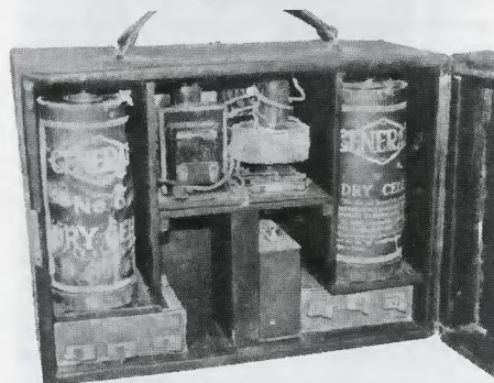
KODEL MODEL P2 — This leatherette portable radio, ca. 1925, uses two Type 199 tubes. There is room inside the case for the A and B batteries, as well as the headphones. (Wally Worth — Wollaston, MA)
