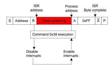
**How to avoid clock stretching**: To avoid clock stretching, measure the Command Program Row (0x39) execution time (Tcom\_ex) according to the system settings (CPU speed, compiler, and compiler optimization level). The host must ask for a response after this time.
