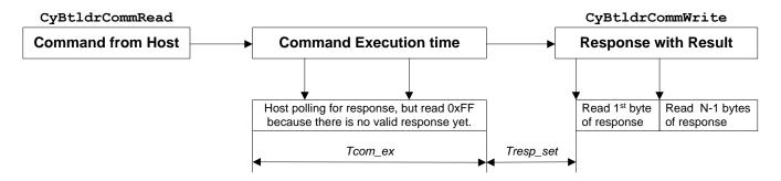
The host must execute polling by reading one byte; reading more bytes could corrupt the response. For example, in the case of 0xFF 0x01 0x03 (two bytes of response were read, instead of one), the next read of the full response returns two invalid bytes, because these bytes were already read (0x01 and 0x03).
