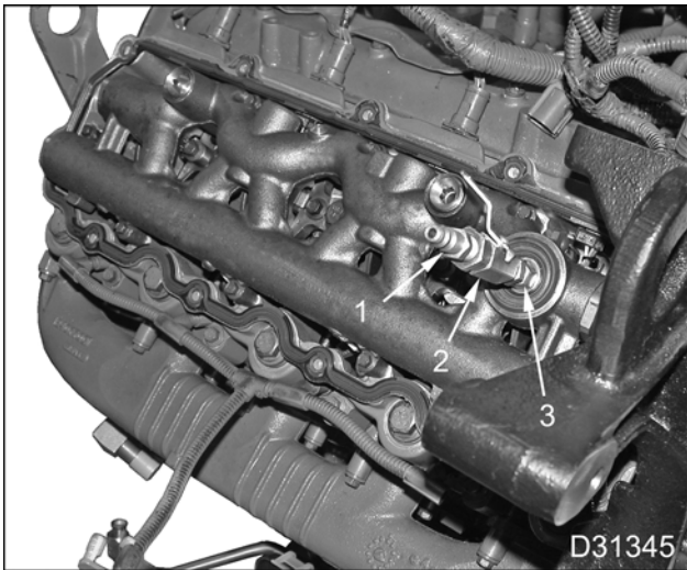
Figure 10 Compressed air supply with valve cover off
