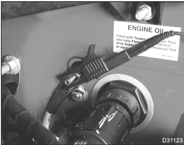
Figure 4 Ground to post on cowl
