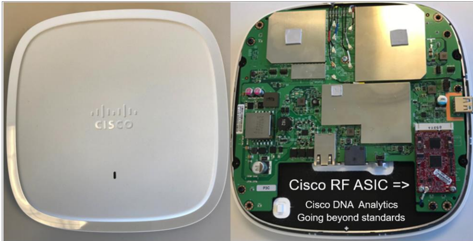
Catalyst 9120i with the Cisco RF ASIC chip
