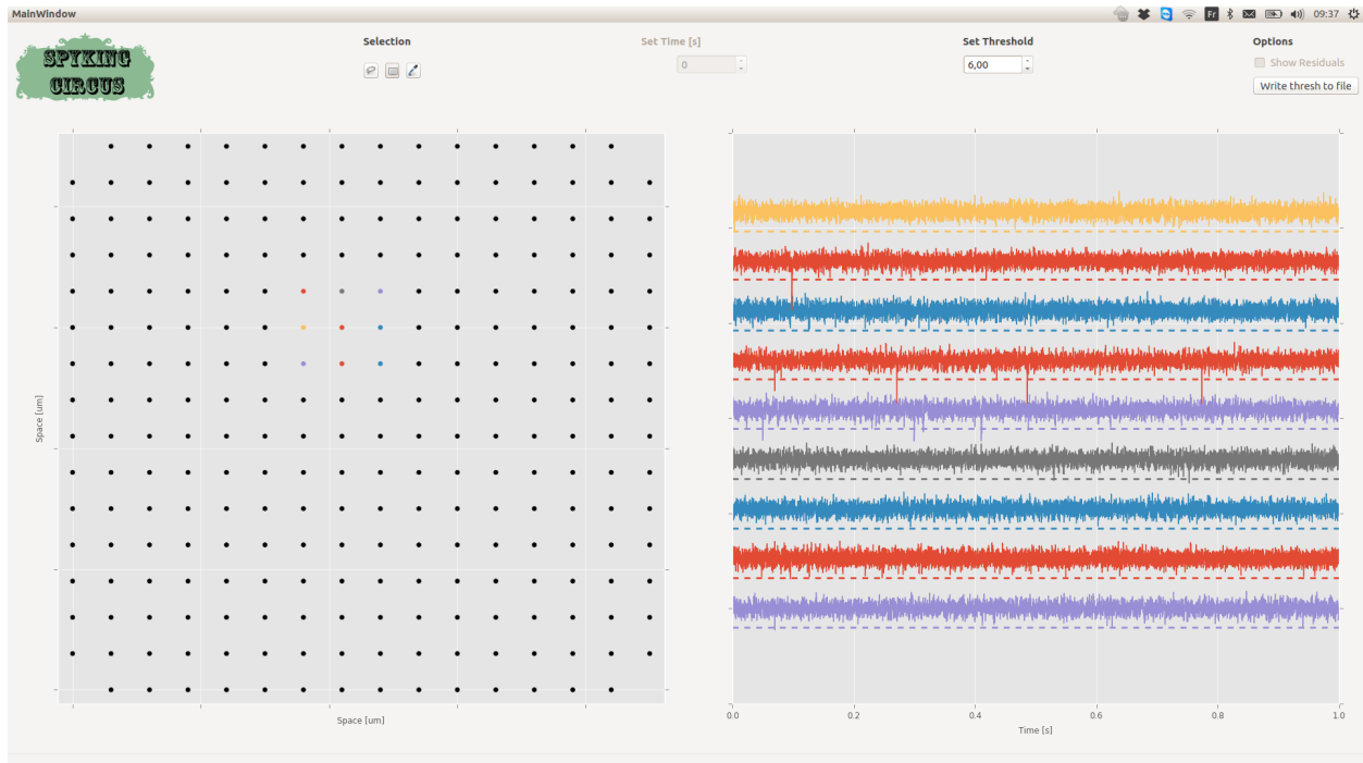
Fig. 2: A snapshot of the preview GUI. You can click/select one or multiple electrodes, and see the 1s of the activity, filtered, on top with the detection threshold
