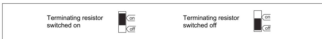
Figure 7-10 Terminating resistor switched on and off
