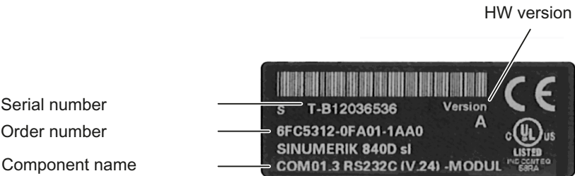
Figure 9-21 COM01.3 RS 232C (V.24) module type plate
