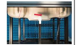
DGBE-based liquids should be used with care. As DGBE is a softener for most plastics, the liquid should be taken out of the phantom, and the phantom should be dried when the system is not in use (desirable at least once a week).
