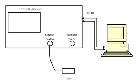
Liquid Verification Setup Block Diagram
