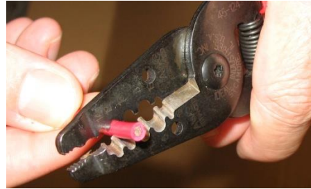
Figure 72. Strip 12 AWG Load Lead Wire
