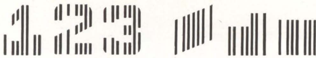
NUMBERS, service symbols and letters are made up of seven vertical strokes of magnetic ink
