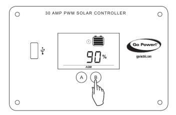
Push the **B Button** to show the battery state of charge (shown as a percentage).
