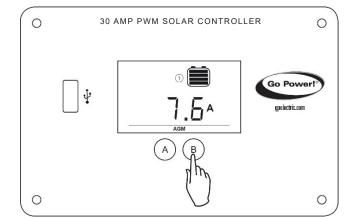
Push the **B Button** to show the PV charging current.
