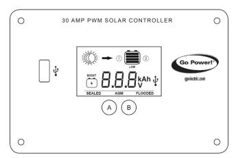
If the GP-PWM-30-SB experiences a battery over voltage (15.5V), the controller will stop operating, and the display will begin to flash with all icons. The controller will resume operating when the error is cleared.
