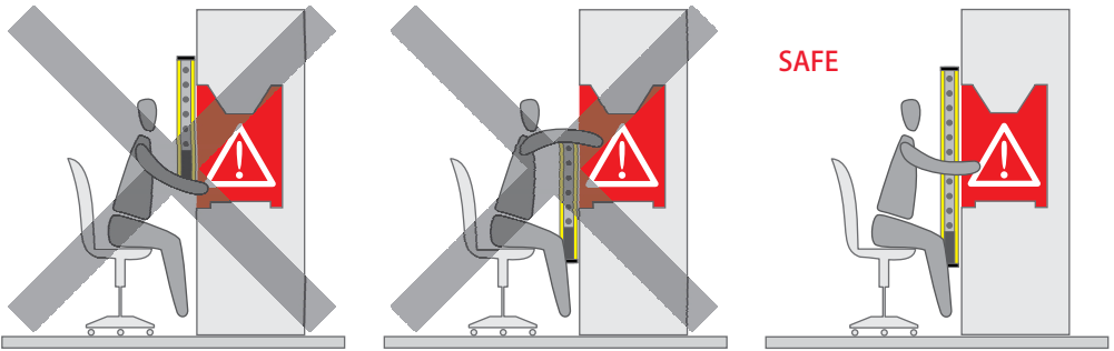
FIG. 9: POSITIONING THE LIGHT CURTAIN
