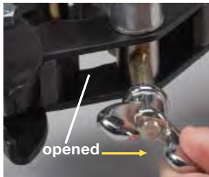
1. With cone up, open the two dies of the clamping yoke
