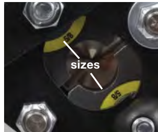
2. Select sizes on underside of dies to match tubing O.D.
