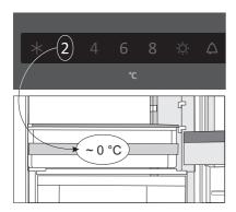
For a temperature around 0 °C in the **ZeroZone** drawer, we recommend setting the refrigerator compartment temperature to less than 4 °C. Temperature in the **ZeroZone** drawer may drop to below 0 °C; therefore, move the food sensitive to freezing to upper parts of the refrigerator compartment.
