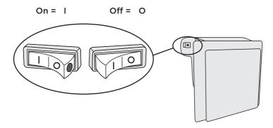
When the ionizer is switched on, a red dot will be visible on the switch.
