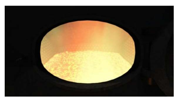
**Coal level average** 60% 1770 *lbs* The grate is covered with the coal's centre on the 3<sup>rd</sup> rivet down on the back wall.
