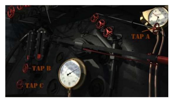
You can also perform blow down tests on the gauge glasses by doing the following:
