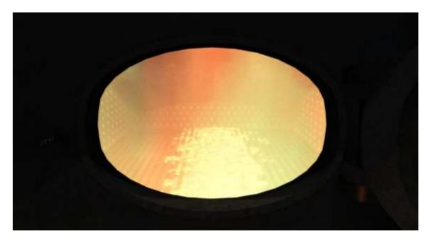
**Coal level low** < 42% 1221 lbs The grate can be clearly seen with a very small amount of coal in the centre.
