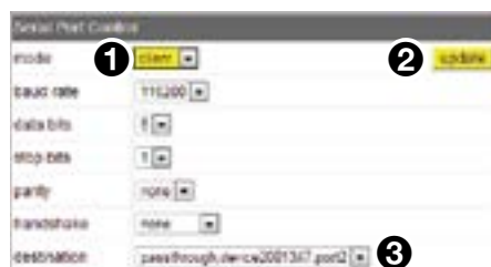
Figure 73. Serial Port Control Panel with Destination menu
