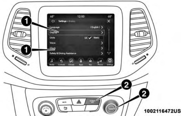
Uconnect 4/4C NAV With 8.4-inch Display Buttons On The Touchscreen And Buttons On The Faceplate
