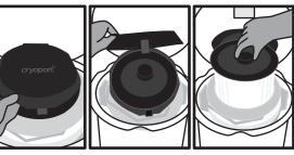
Open the hinged cap by pulling up on one of the two lift handles on the lid. With gloved hands, pull up on the circular handle in the center of the vapor plug to remove the vapor plug. Set the vapor plug aside.
