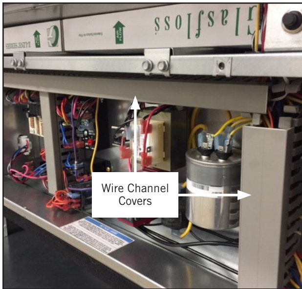
FIGURE 9 Remove Wire Channel Covers
