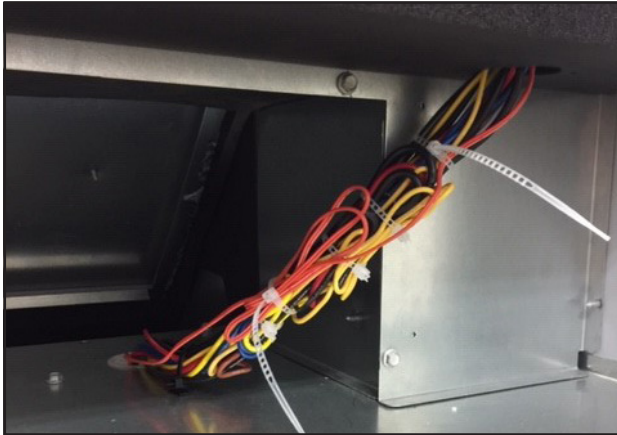
FIGURE 12 Pull Wire into Exhaust Area and Fasten with Ties
