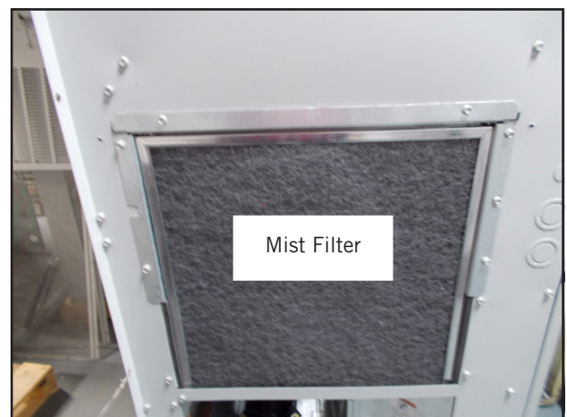
FIGURE 19 Install Mist Filters
