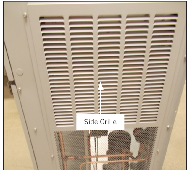
FIGURE 2 Remove Side Grilles
