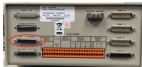
Figure 3: USB cable 68-1247-504, wiring, and plug location on controller rear panel
