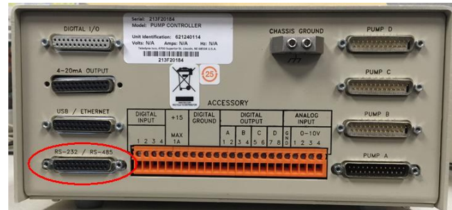
Figure 2: Serial Cable 480-7996-00, cable wiring, and plug location on controller rear panel
