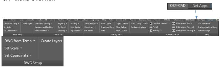
The DWG Setup section of the OSP-CAD menu is used for creating New Drawings, Setting Scale, Setting Coordinate and Creating Layers.
