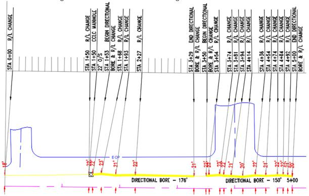
h. Everything you see above was created by the "Place Object" program. After the user has finished drafting the cable line the polylines will need to be joins (excluding the Directional Bores) in order to display the line type correctly.
