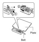
Pass the end with the ◀ mark of the reflector adapter's belt through the plate (①) and insert the ◀ part of the belt into the plate (②).
