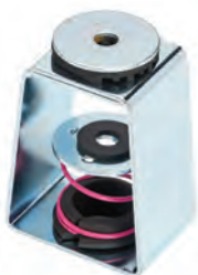
CH30SCS Type Deflection Combination Hanger 15° Tilt Spring & Neoprene w/ Seismic Cushion Stop 1" & 2" Deflection Pages 285 & 286
