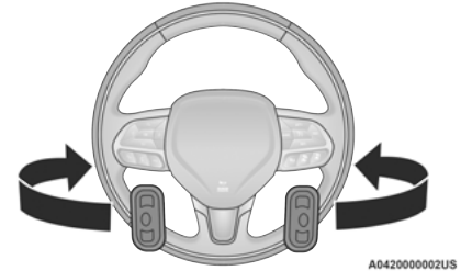
Remote Sound System Controls
