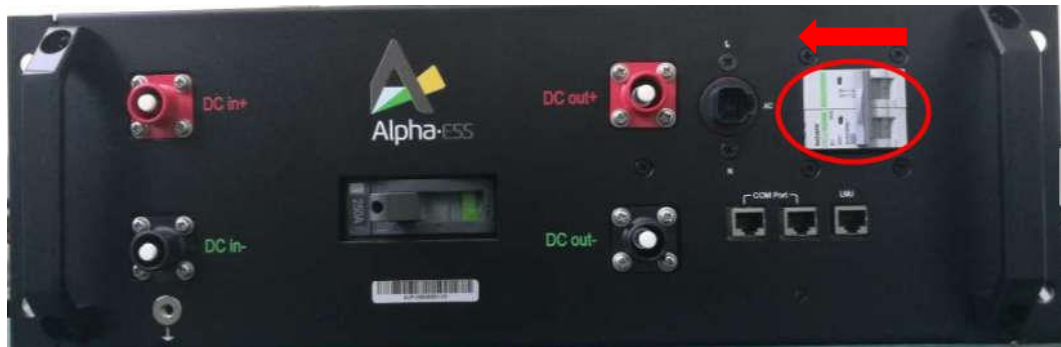
Figure 5.2 AC switch in switch-on status
