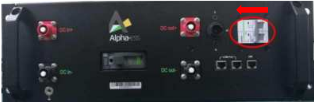
Figure 5.2 AC switch in switch-on status
