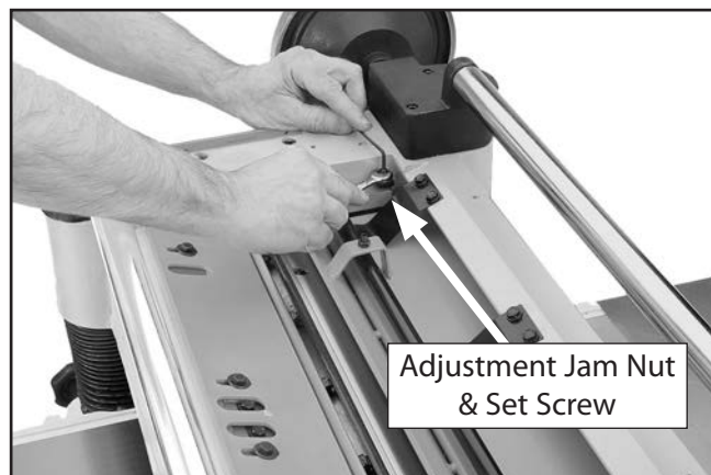
Figure 57. Example of adjusting the pressure bar height.
