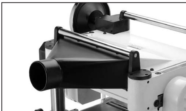
Figure 16. Dust hood installed.
