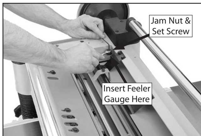
Figure 61. Feeler gauge location for adjusting pressure bar height when using wood blocks.
