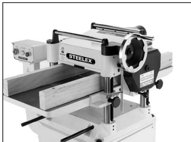
Figure 58. Gauge boards installed.
