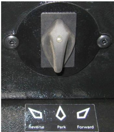
Figure 14: Drive Selector Switch
