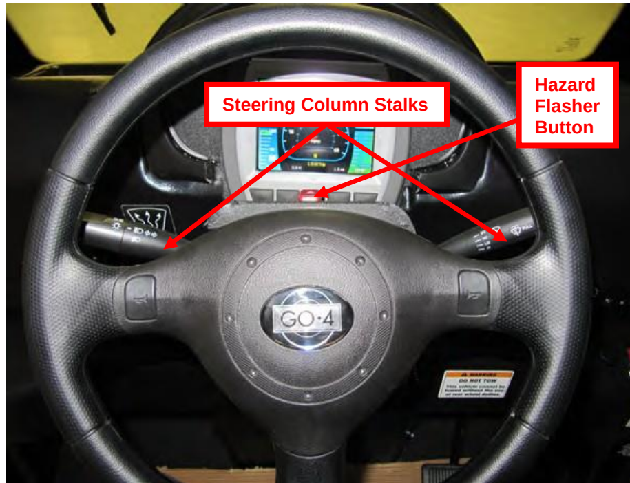
Figure 20: Steering Column Stalk and Hazard Flasher Button Locations
