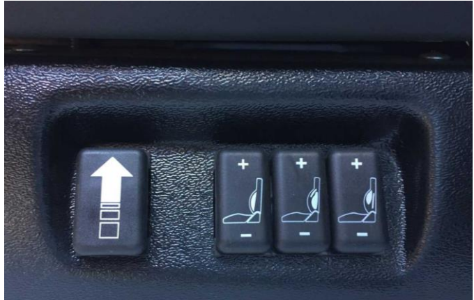
Figure 27: Power Seat Controls (Height, Bolstering, Lumbar)
