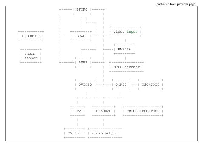
The GPU is made of:
