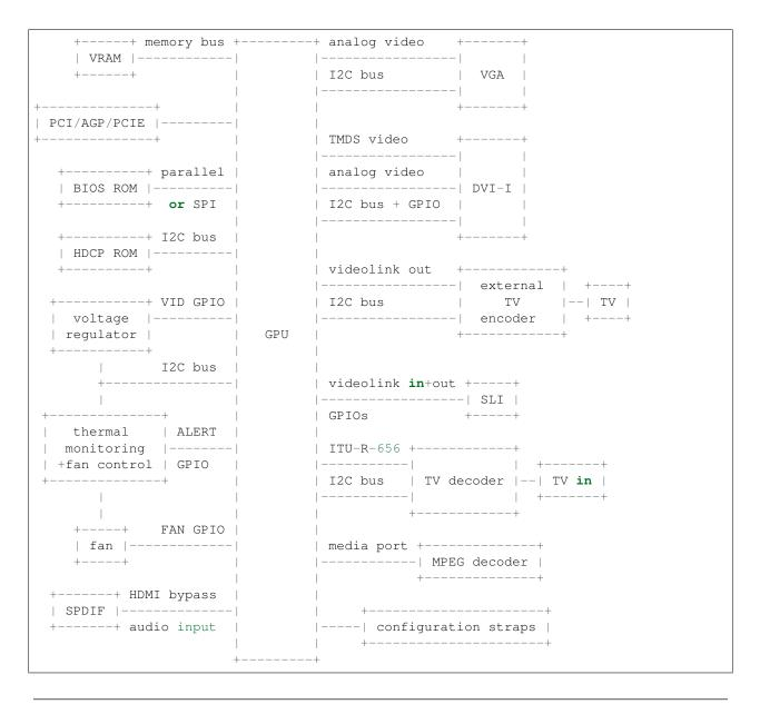
**Note:** while this schematic shows a TV output using an external encoder chip, newer cards have an internal TV encoder and can connect the output directly to the GPU. Also, external encoders are not limited to TV outputs - they're also used for TMDS, DisplayPort and LVDS outputs on some cards.
