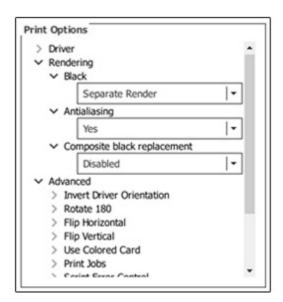
Black - configures how the black color is sent to the printer. You can **Send as RGB**; **Send as Monochrome**; **Send as RGB and Monochrome**; **Send Composite**; **Send Composite** and **Monochrome** or send as a **Separate Render** (default option).
