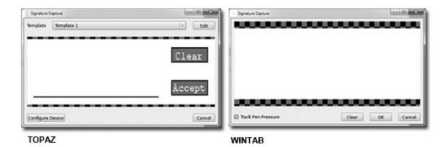
The Topaz device also allows you to have templates for the signature frame. The Wintab driver has a track pressure setting that according with the pressure made by the pen, makes the line thinner or thicker.
