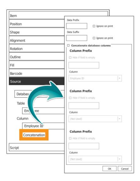
**Concatenation** allows you to stack up to three database fields within the same **Barcode**. This is allows for a much more dynamic and space efficient data generation when working with barcodes.
