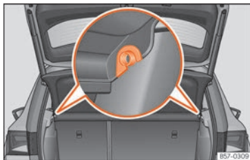
Fig. 116 In the luggage compartment: removing and fitting the shelf.
