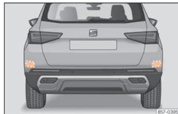
Fig. 160 Rear view of the vehicle: radar sensor zones.
