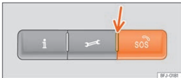
Fig. 30 On the roof console: voice service controls
