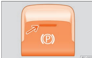
Fig. 182 In the lower part of the centre console: electronic parking brake button
