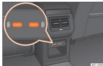
Fig. 147 Rear part of the centre console: USB connectors with power outlet function. »
