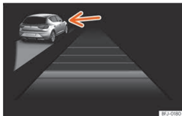
Fig. 170 On the instrument panel display: ACC active, vehicle detected in an outer lane.
