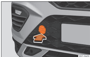
Fig. 45 On the right side of the front bumper: remove the cover.
