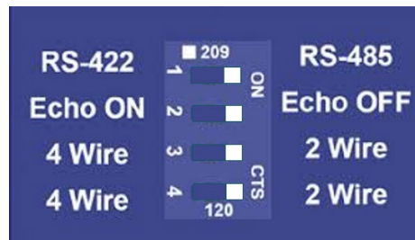
Figure 11: Dip Switch settings
