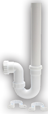
ZB33056DB P-Trap 76mm seal 40mm 600mm upstand pipe
